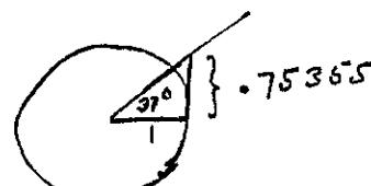
The Table of Tangents is one of the three tables commonly used in trigonometry. The other two are sine and cosine.
