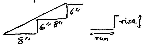
For our stairs, rise divided by run =  $6 \div 8 = 0.75$ . In the table we see .75355 which is nearly the same as 0.75. This tells us that the plank would make an angle of, very nearly,  $37^\circ$ .
